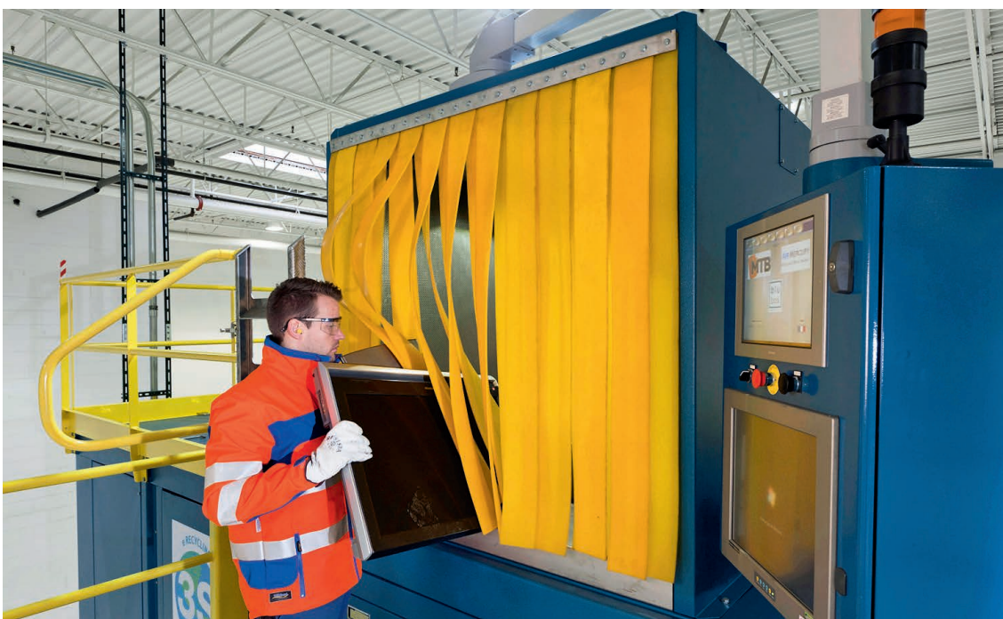
▲ A large flatscreen is fed into the shredder
