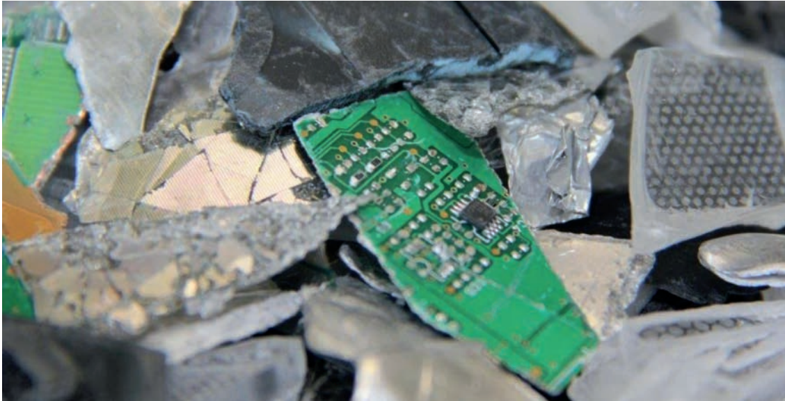
◀ Downstream fraction leaving the shredder: a mix of printed circuit boards, plastics, LCD glass and PMMA
